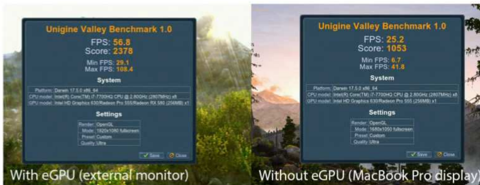
Benchmarks from a 15-inch 2017 MacBook Pro using Unigine's Benchmark Valley on Ultra (fullscreen), both with the eGPU and without.
